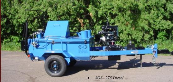
Used for melting and applying crack sealing materials for asphalt and concrete road surfaces.
