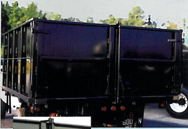
Flatbed with removable metal sides and barn door. Also close up view of barn door latch
