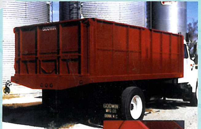
Inside Pocket Body with 48" plywood grain sides and swinging tailgate with grain door
