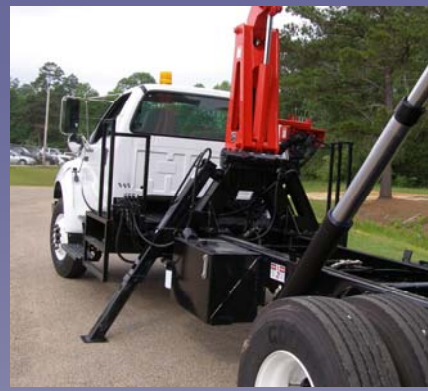
Low profile pedestal with "A-Frame" outriggers. The outriggers extend to a width of 9 ½ feet.
