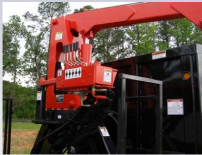
Controls swing from side to side for operator requirements. Optional dual controls available.
