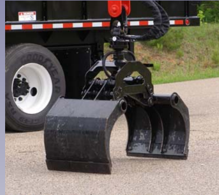
The boom is equipped with a continuous rotating grapple. The grapple is constructed with bolt-on heat-treated steel cutting edges for ease of replacement. The edges are overlapping to prevent scalping. The bucket is 36" wide with a 48" opening from lip to lip.
