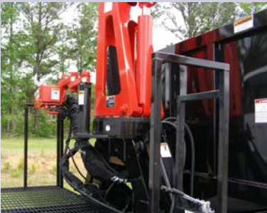
Controls swing from side to side for operator requirements. Optional dual controls available.
