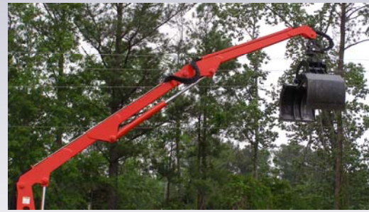
The boom is a 17 foot fixed boom constructed with a one piece main boom.
