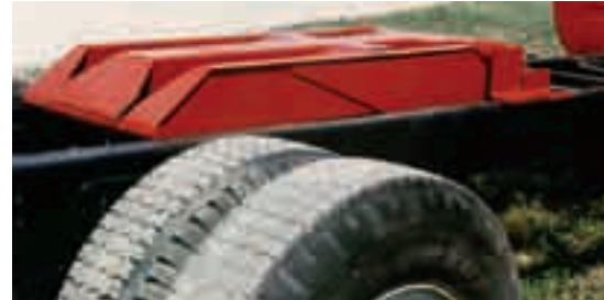
Hoist mounts low between the frame, meaning no notching crossmembers under dump body.
