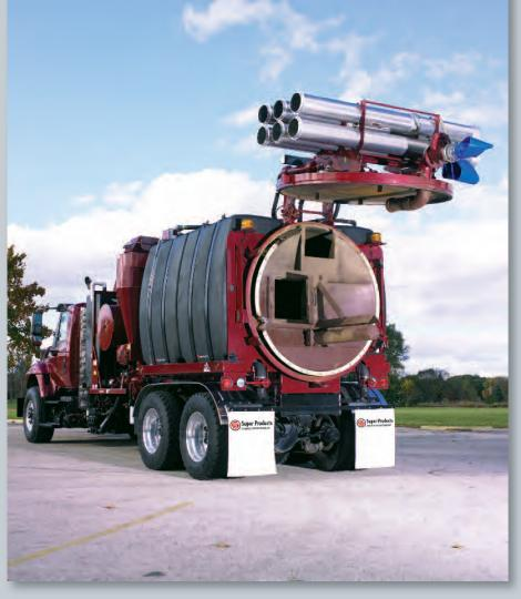
From its ejector plate unloading and dewatering system to its water recycling capability, Super Products' Camel sewer and catch basin cleaner is truly unlike any other combination unit on the market today!
