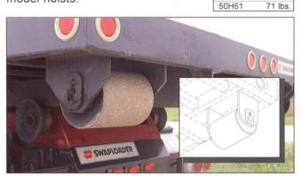
Container/truck body Roller Assembly for use with all sub-frame sizes. Roller mount Brackets also shown.
