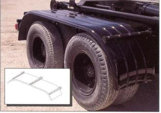
Tandem Axle Fender, steel, fits tire sizes 22.5" to 24.5". Includes mounting brackets.
