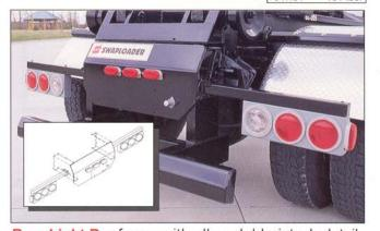
Rear Light Bar foruse with all model hoists. Incl. tail, brake, backup, license plate, side and rear clearance lights, mount brackets.
