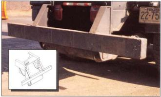
Truck rear end **Stabilizer** for use with SL-405 and larger hoists. H.D. bumper incorporated into design. Shown in travel position (photo) and lift position (drawing).
