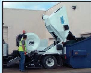
The easy to open hydraulic dump door lets you dispose of bulky items quickly and safely into most 6 and 8 yard dumpsters or containers. The Hopper Drip Edge Extension extends reach for cleaner dumping.
