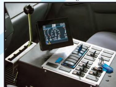
**In-cab controls** are center mounted and illuminated for ease of operation from either driving position. Switches integrate multi-color LEDs giving operators instant feedback on sweeper functions.
